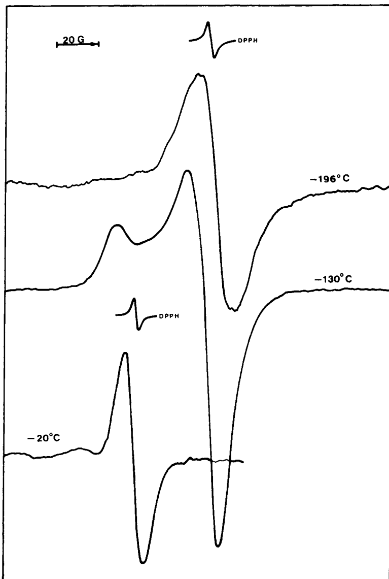
Fig. 4. ESR spectrum as function of temperature of polyethylene (HDPE ELTEX A 1050) activated by DPPH, after 25 hr of indoor aging in air (xenon lamp, \lambda > 290 nm).
